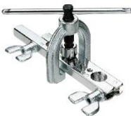
Flaring Tool Set Item : FT-10A Capacity : 3/16", 1/4", 5/16", 3/8", 7/16", 1/2" & 5/8"
